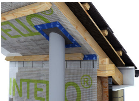
Above: A pro clima service grommet sealing a pipe penetration of the airtightness layer (left); A “service batten” on the inside of the INTELLO PLUS which reduces likely service penetrations of the membrane (middle); Overlaps of the Intelligent vapour check, INTELLO PLUS, sealed at critical junctions with pro clima airtight system proprietary seals (right)
